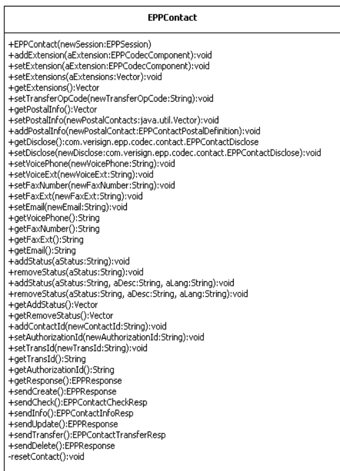
Figure 11 - EPPContact Class Diagram
